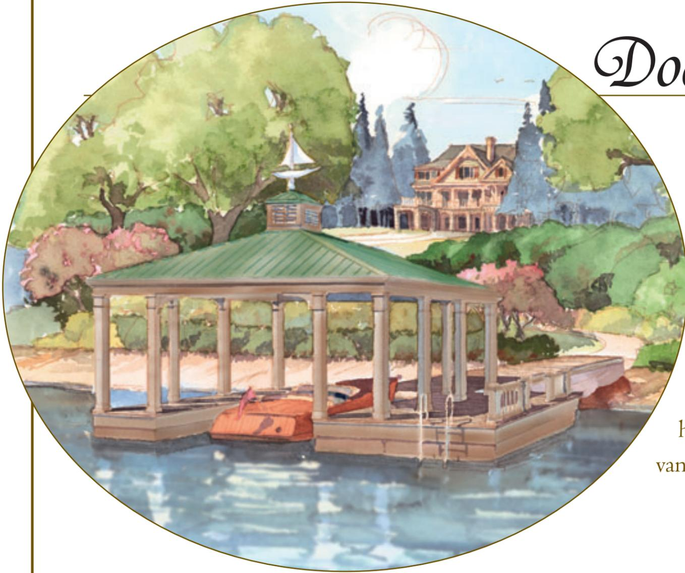
Docks at Keowee Falls South must conform to the standard design guidelines for the community. All vertical members must be wrapped with traditionally detailed materials and match the design style established for Falls South. The dock roofs will be a uniform forest green standing seam metal to blend the building with views of the lake from home sites above. A cupola and weather vane are standard features.
