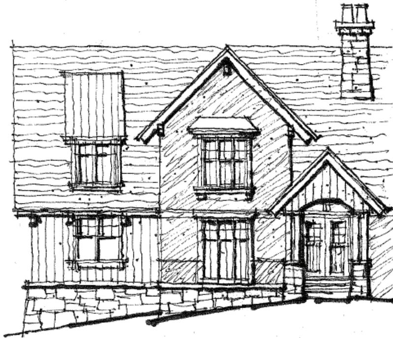
Low E glass is acceptable and encouraged where solar glare and heat gain are a problem. All windows in a stone, masonry or stucco veneered wall must have a lintel comprised of stone, wood or masonry. Windows requiring jack arches shall use pre-cut or machine-cut brick or stone.
